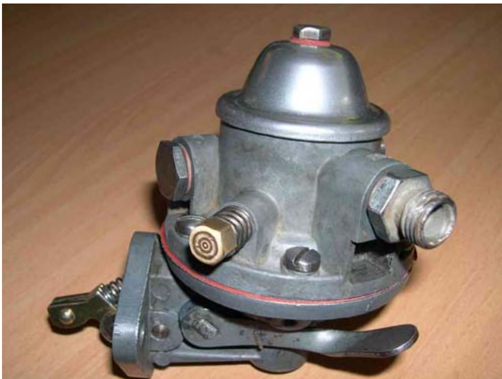
Completed fuel pump
