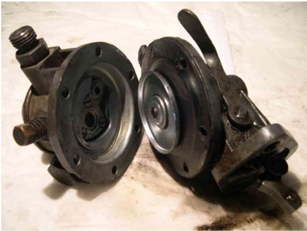
Pump body separated showing original diaphragm
