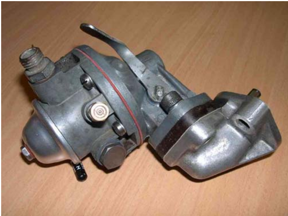
Pump and bracket together and completed
