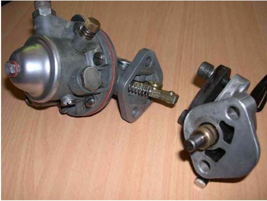
Pump and engine bracket before bolting up
