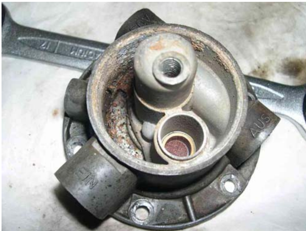
With filter removed, a lot of debris is visible
