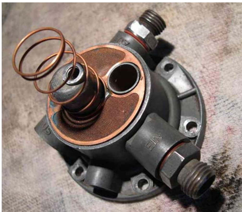
New filter and spring in cleaned up housing
