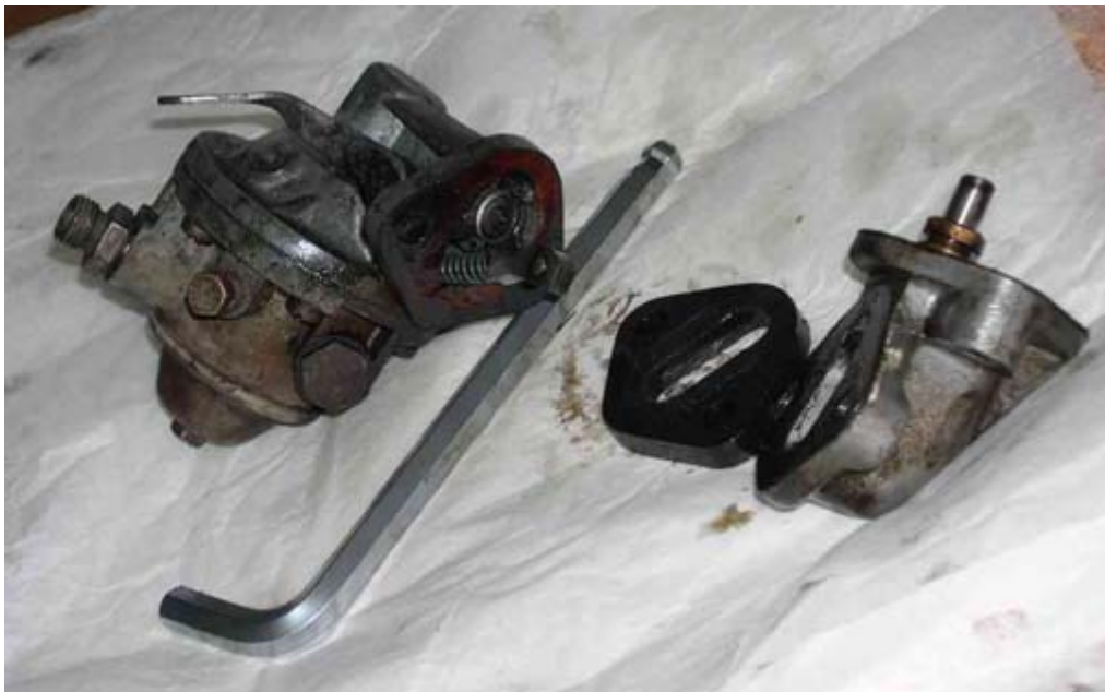
Pump and bracket separated &MDASH; Note cam follower at top of bracket
