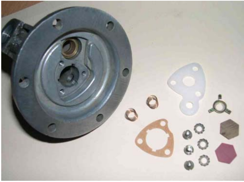
New valve parts showing hard white plastic item 15
