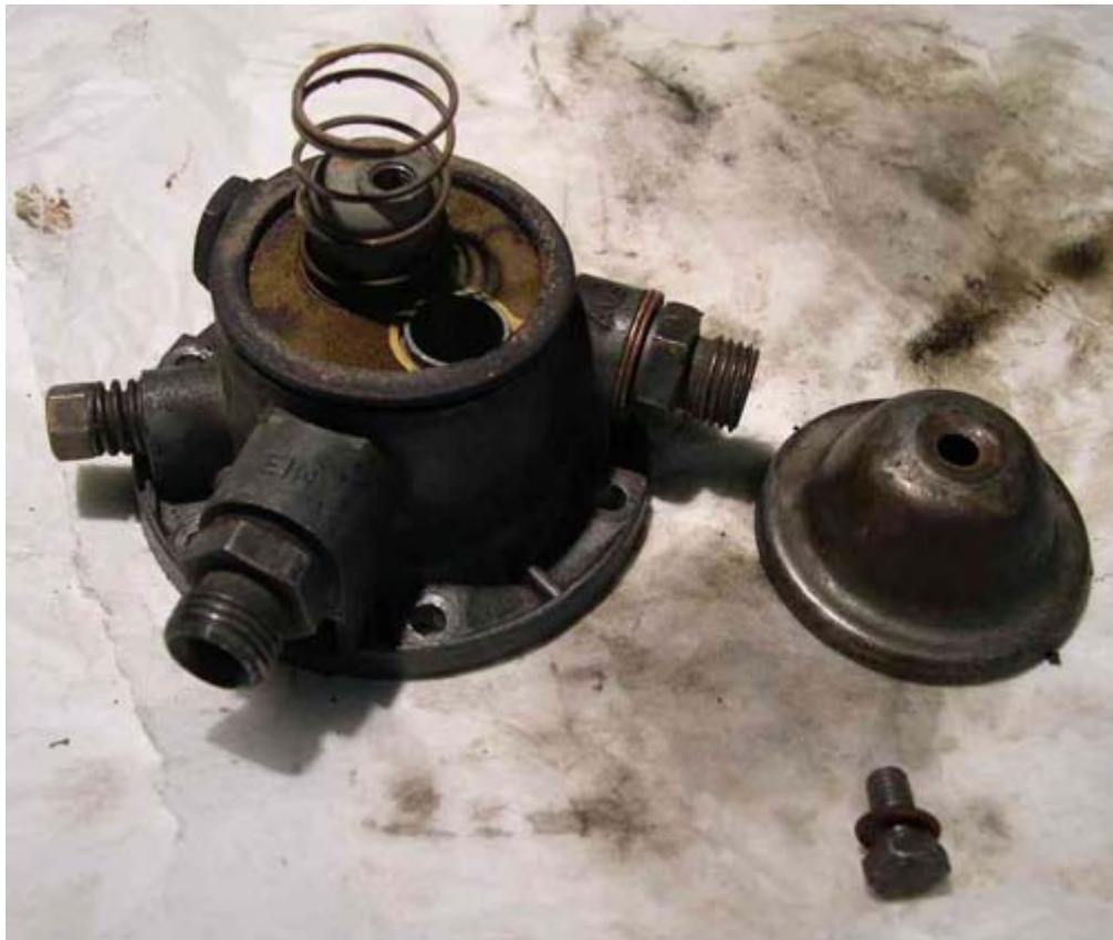
Filter cap removed showing original filter and spring inside
