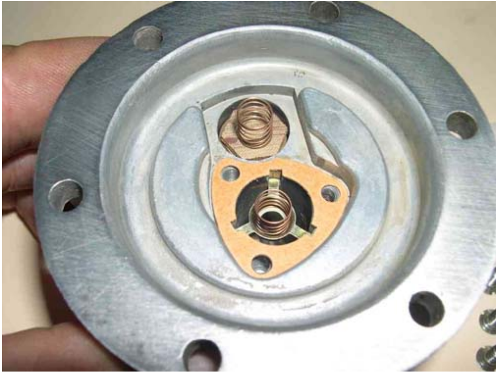
Valve springs, valves and gasket in place
